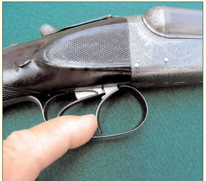
One of the Westley's most intriguing features is an articulated front trigger.
